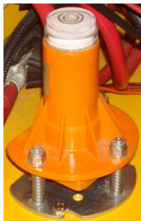
Figure 4-11. Level Sensor Pendulum Based
